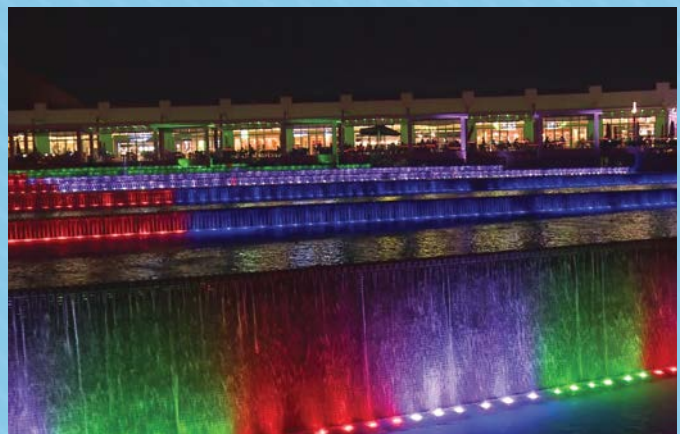
The water fall weirs were illuminated with Aquashi stainless steel LED 30 watt 24v, RGB lighting that provided multi colour lighting effects to the weirs
